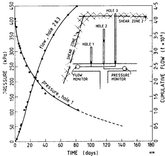
Fig. 4.- Gas pressure and gas flow from shear zones.
