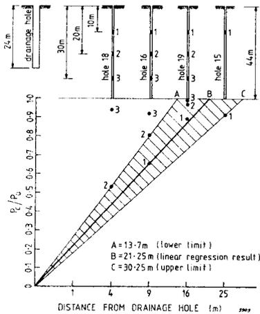
Fig. 11.- Effect of sphere of influence of a drainage hole.
