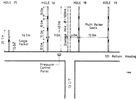
Fig. 10.- Arrangement of test to determine sphere of influence of a drainage hole, West Cliff.
