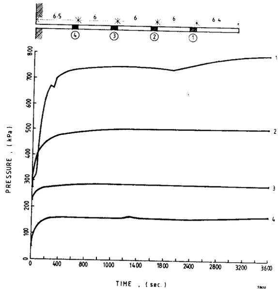
Fig. 8.- Pressure build-up as a function of time using a Quadruple packer system. Hole 33, Panel 121, length of hole 40.5 m, seals placed at 76.5 m from collar of the hole, with 6 m chambers between the seals, inflation pressure 13000 kPa.
