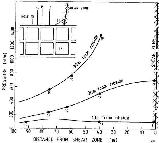
Fig. 3.- Gas pressure changes close to a shear zone.
