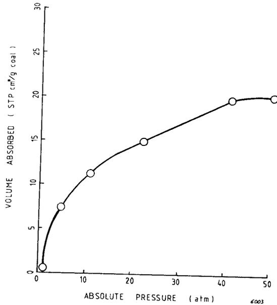
Fig. 7.- Methane adsorption in coal at high pressure, Panel 304, West Cliff Colliery (Temp.  $20^{\circ}\text{C}$ ). Courtesy Intercomp, U.S.A. 1979).
