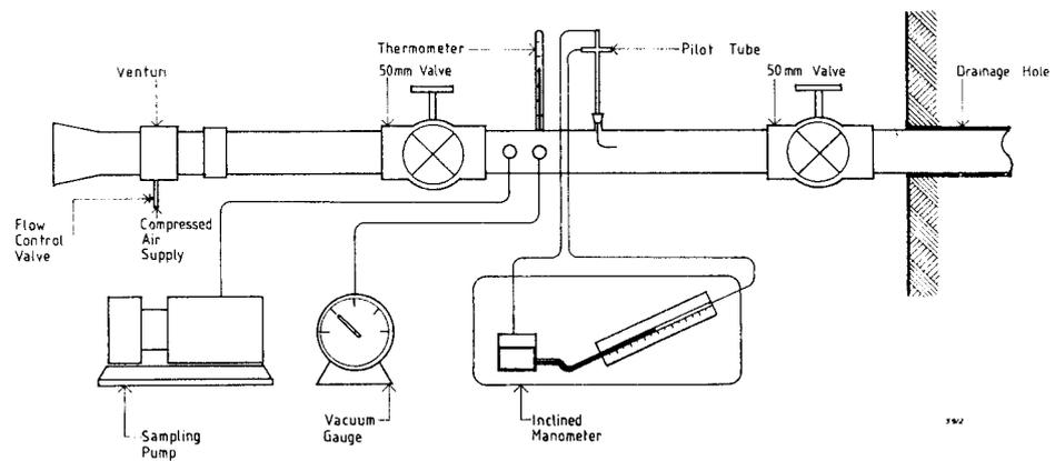
Fig. 14.- Schematic arrangement for testing drainage holes under suction.
