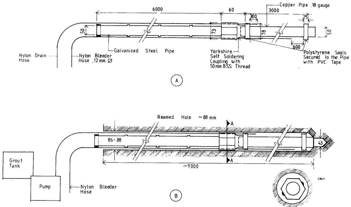
Fig. 9.- (A) standpipe ready for grouting; (B) standpipe grouted in hole using a grouting pump.
