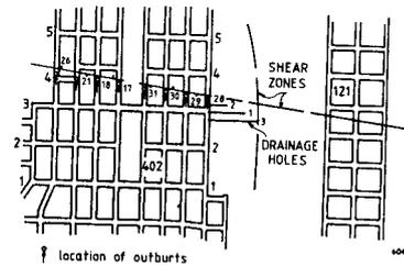
Fig. 6.- Layout of Panel 121, shear zones and drainage holes.
