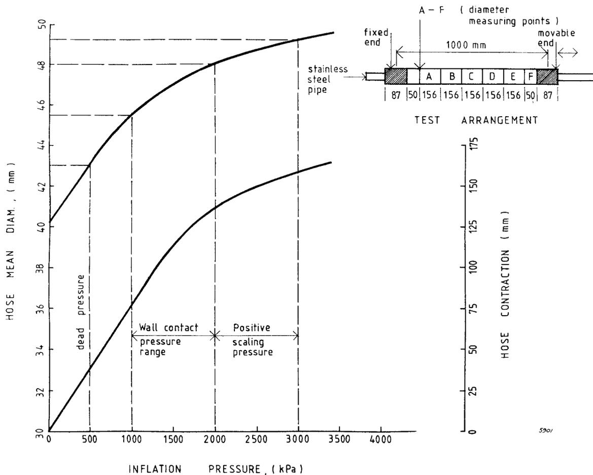
Fig. 2.- Inflation characteristics of petrometallic dilatible hose, 1 m in length.
