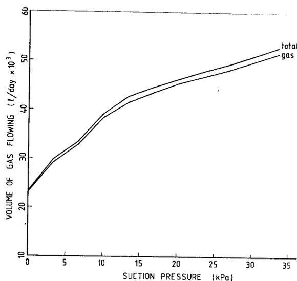
Fig. 16.- Influence of suction on flow of gas from borehole 304-29, drilled on 4/12/79, tested on 12/12/79, depth 90 m.
