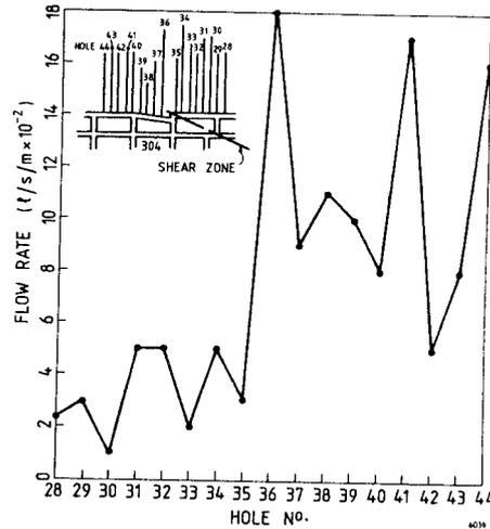
Fig. 5.- Gas flow rates from holes and location of shear zones.
